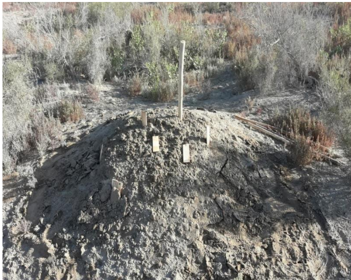
Figure 1. Installation in the termite nest of wood samples soaked in an aqueous solution of the chemical drug "Piralax - Lux" in the termite nest under natural conditions
